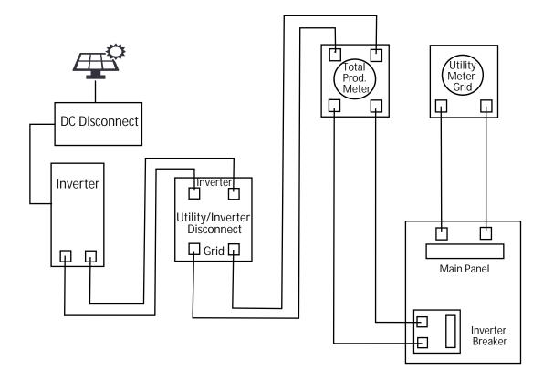
Note: Solar systems that that are energy storage (battery) do not require a production meter.
